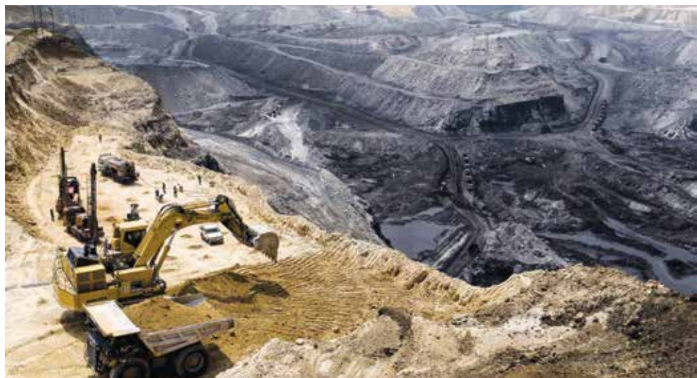
An excavator loads soil onto a truck at an open coal mine near Mahagama in Jharkhand.
