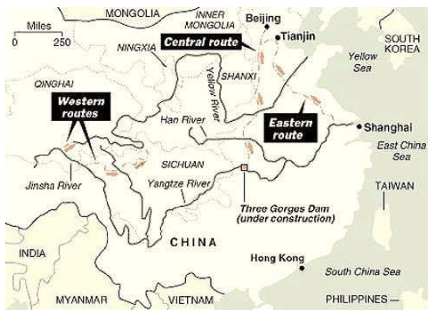
South-North water Transfer Project: image Courtesy water-technology.net
