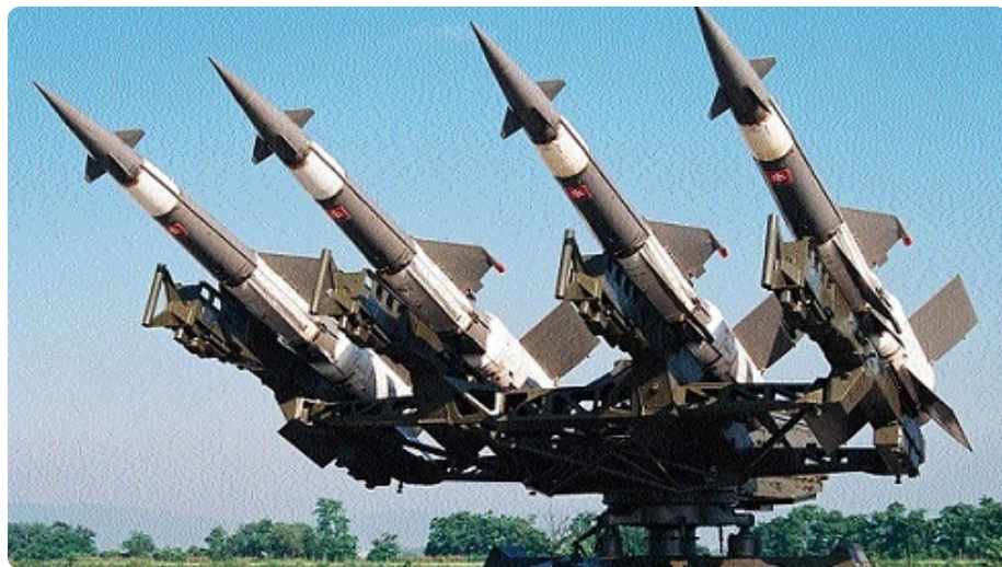
The Russian SA-3 Pechora Surface to Air Missile, Deployed 5P73 four rail launcher (images © 2009, Miroslav Gyürösi). (representational image)
